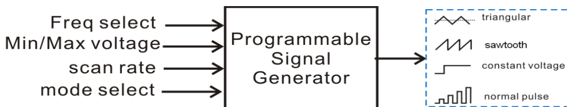
Figure 2: The function schematic of the programmable signal generator.
